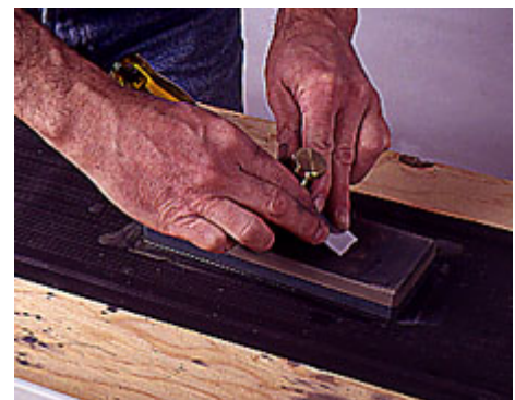
5—Once a uniform bevel is created on the blade edge, turn over the stone and finish sharpening on the fine side.
