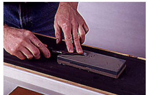
1—Begin sharpening a chisel by flattening the back of the blade on the coarse side of the waterstone.
